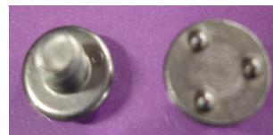
**JPGW Series - This Flange Weld Stud with 3 projections on top of the flange enables welding the stud to the surface, as opposed to through the material. Made from a high-welding quality low carbon steel.**
