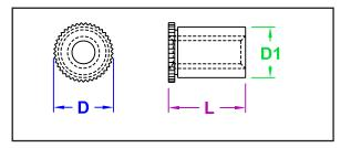
CF40 & CF40S miniature standoffs are designed to be used in limited space applications. They are ideal for securing D-sub connectors to enclosure backplanes and provide a flush mounting surface for RFI/EMI gaskets.
